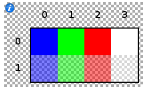
Example 2 of a 4×2 pixel bitmap, with 32 bits/pixel encoding
